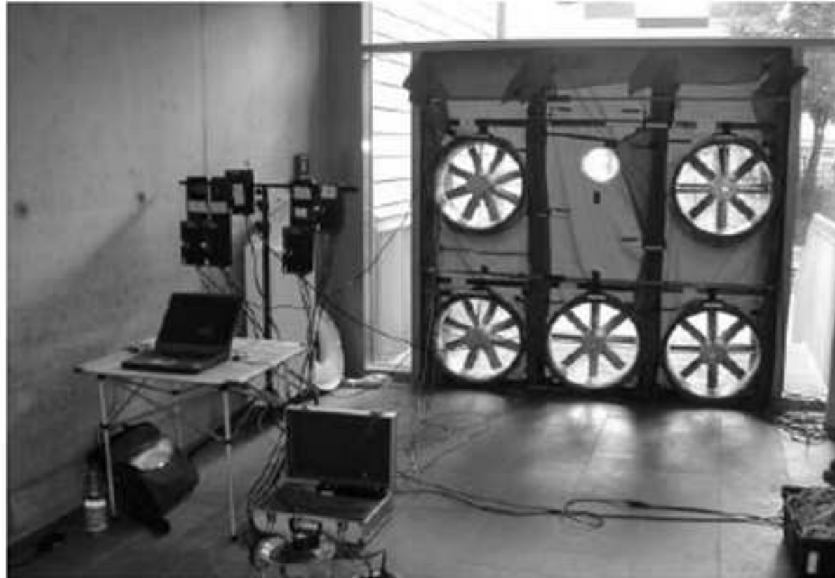
Fig. 6: Central installation of the measuring equipment (Source: IngBEU)
